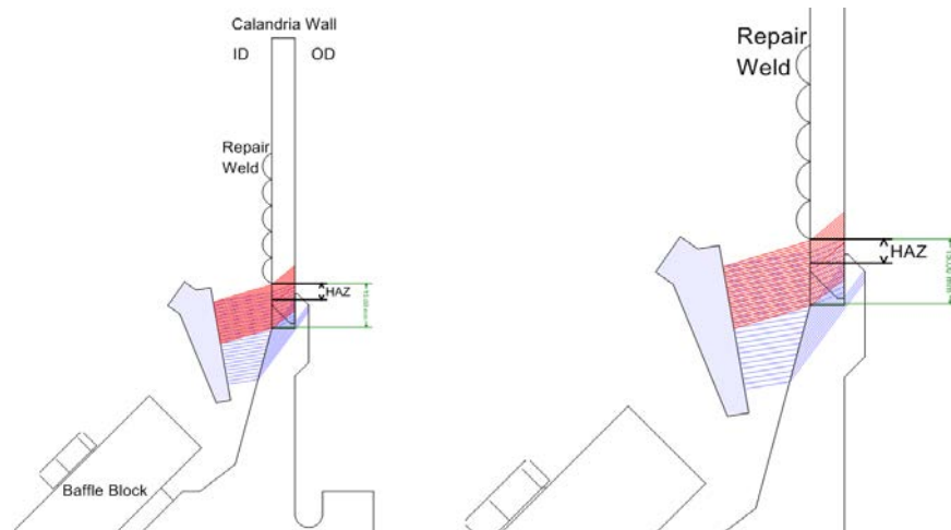
Figure 6. Lower HAZ technique: Overview and detail
